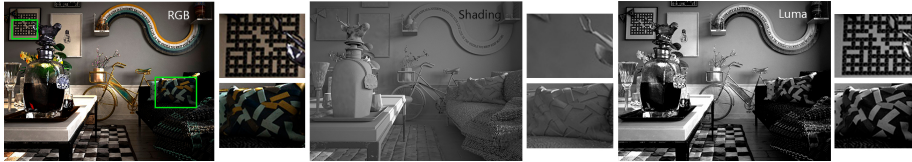
Fig. 5: We show the difference between the shading representation and the L-channel from LUV. The shading correlates well with the geometry, while the L-channel includes texture information as shown in the green insets.
