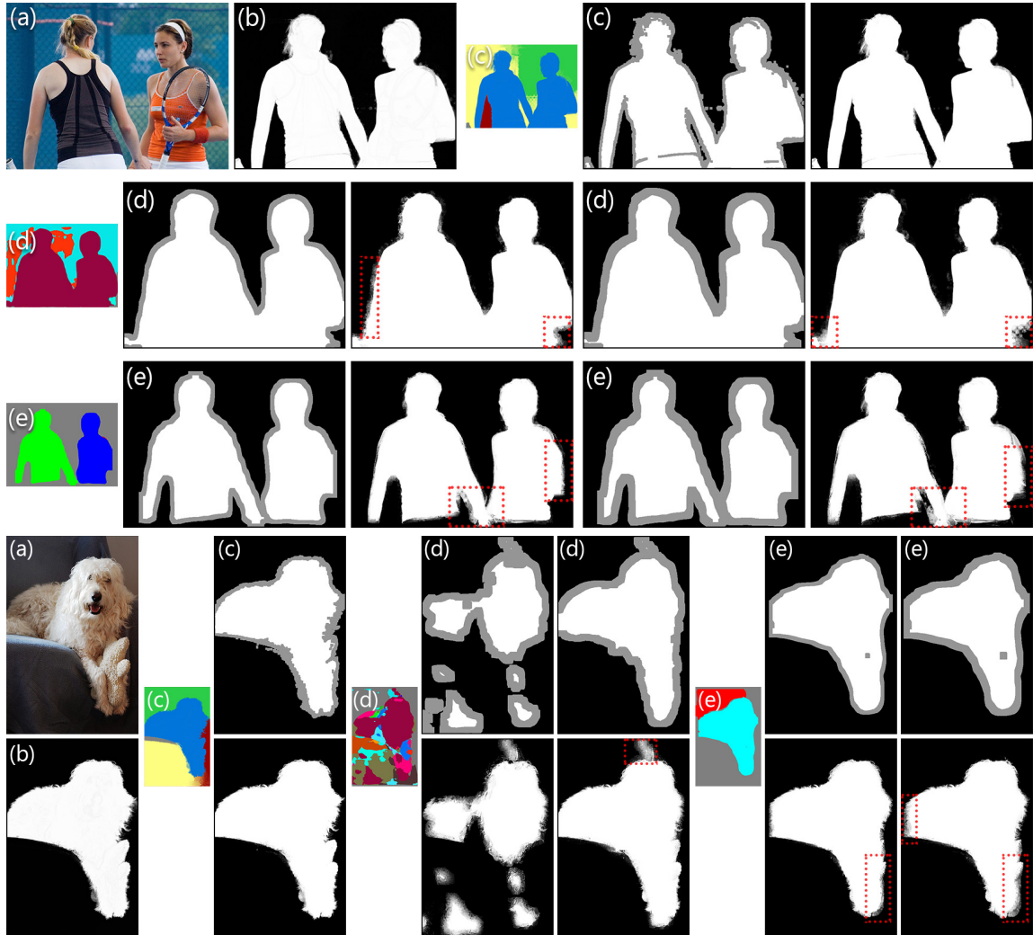
Figure 6.12.: From the input image (a), our method generates the matte shown in (b). We show that the trimaps with different unknown region widths, generated using the semantic segments by PSPNet [Zhao et al., 2017] (d) or Mask R-CNN [He et al., 2017] (e), fail to provide foreground and background regions reliably, which affects the matting result generated using information-flow matting Chapter 5 negatively. In the bottom example, PSPNet trimaps are generated by selecting a single class (left) or all the classes that correspond to the object. We also provide the matting result using a trimap generated by our result (c) which demonstrates the performance of the matting algorithm given an accurate trimap. Images from [Lin et al., 2014].
