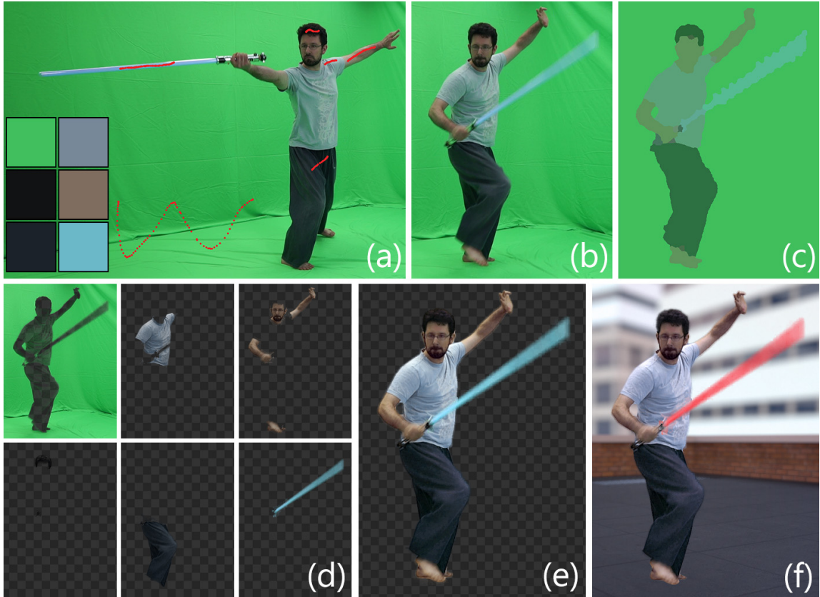
Figure 3.1.: Major steps of our method. First, parameters of a global color model are obtained from a key frame via a simple scribble interface (a) (Section 3.2.1). For a different query frame (b), the global color model is refined into local color models (c) (Section 3.2.2) which are utilized for extracting multiple color layers via color unmixing (d) (Section 3.1). A subset of layers is then combined to get the final keying result (e). The layers can be used for compositing as well as color editing (f).
