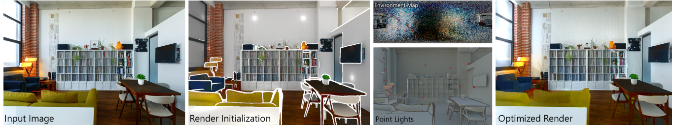
Fig. 1. Visualization of our lighting optimization process. For a given input image, we first extract the diffuse-only image using CID. We then initialize an environment map and a grid of point lights in Mitsuba. We optimize the values of both the environment map and the point lights. The third column shows the optimized environment map, and point light positions visualized as red spheres. The last column shows our rendered version of the scene after optimization. Image from Unsplash by Nathan Van Egmond
