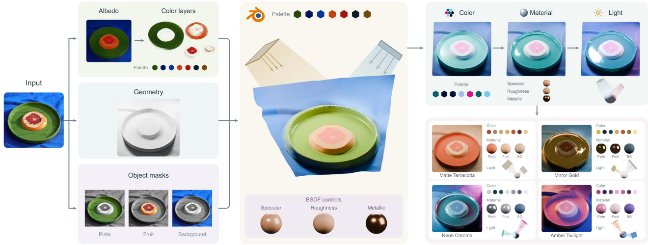
Figure 2: Our pipeline: intrinsic decomposition [Careaga and Aksoy 2024] followed by soft color segmentation [Aksoy et al. 2017] gives a palette and per-pixel alpha maps; MoGe [Wang et al. 2025] estimates geometry; and SAM 2 [Ravi et al. 2025] produces per-object masks. Then a Blender scene with Principled BSDF shader graph that exposes color, material, and light controls is created. Each component is then exposed for the user to edit. Image credits: @Mustafa akın
