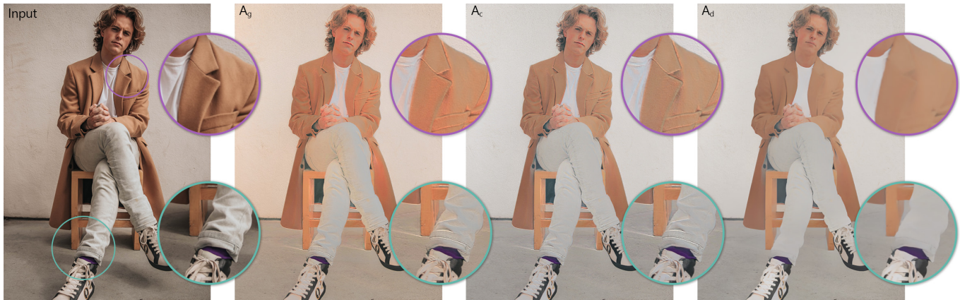
Fig. 4. Our pipeline is able to iteratively correct small errors in at each stage. In this example, our pipeline first corrects the colors on the folds of the clothing when estimating shading chromaticity. Then the albedo estimation network is able to remove small errors from the original decomposition by estimating a smooth albedo layer. Images from Unsplash by Austin Wade.
