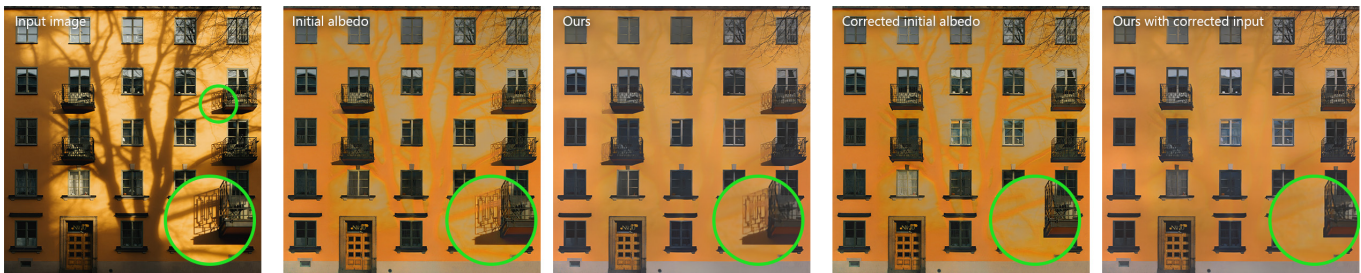
Fig. 12. As our pipeline starts with a grayscale intrinsic decomposition as input, it may not be able to fix strong mistakes made by the initial model, such as the hard shadows of the balconies incorrectly included in the initial albedo on the left. However, we show that these mistakes can be fixed when the input albedo is corrected, in this case using Photoshop’s content-aware inpainting tool.
